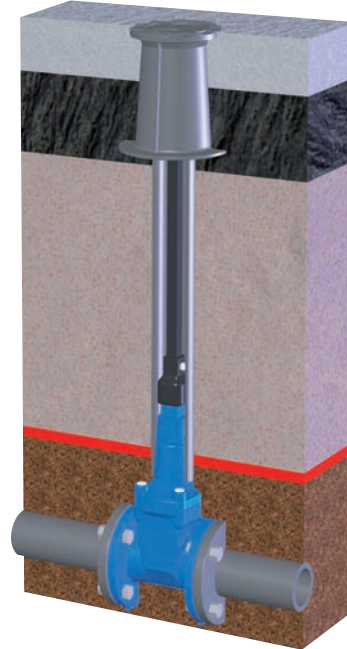
Installation de vanne enterrée Installation of buried gate
