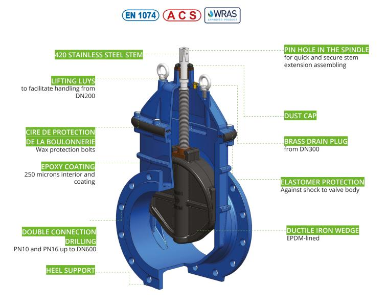
$\checkmark$  Corrosion Resistance: the valves are 250µm epoxy paint coated on the outside and inside of the body and the bonnet.
